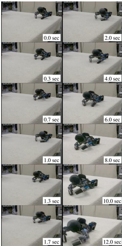
Fig. 3. Crawling motion executed by the developed platform.
