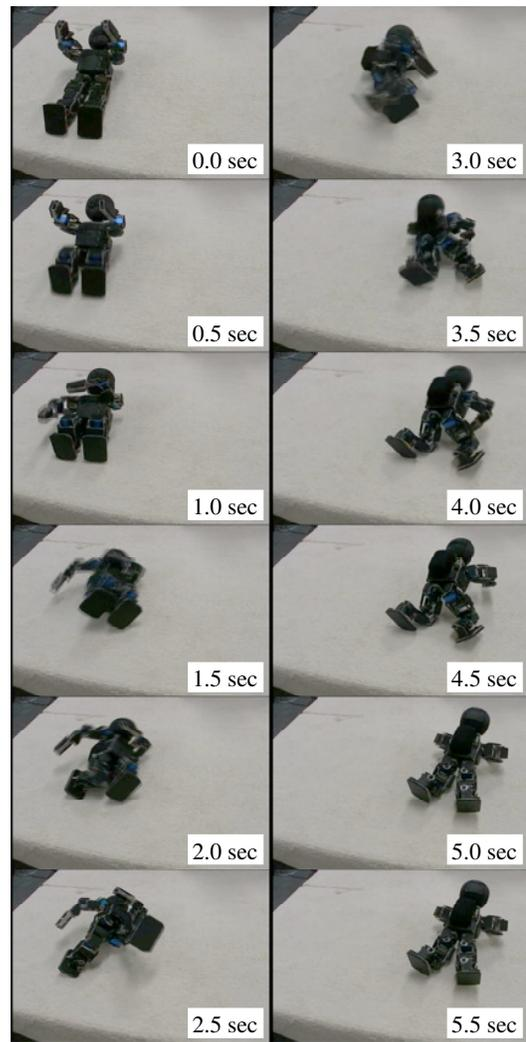
Fig. 4. Turn over motion executed by the developed platform.
