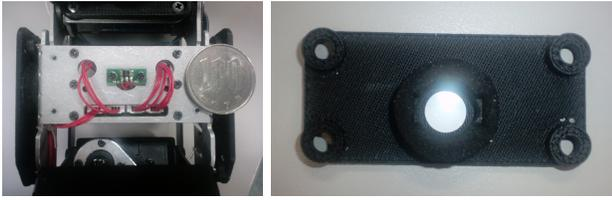
Fig. 5. Photo of the photo interrupter board attached to the robot's aluminum frame and plastic plate
