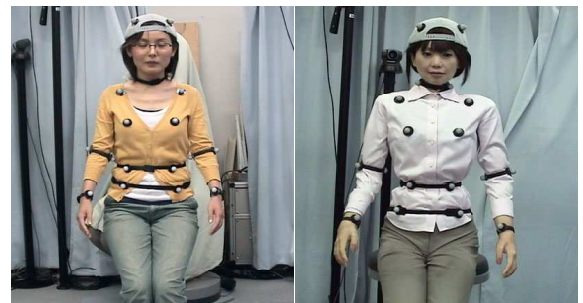
Fig. 5. The subject's postures mapped onto the android (discouraged, \delta_e = 24.9\text{mm} , \sigma_s = 6.3\text{mm} ).
