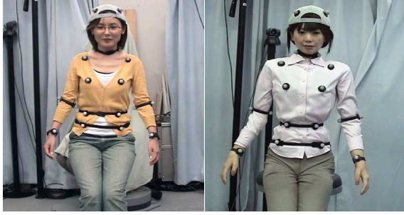
Fig. 7. The subject's postures mapped onto the android (avoiding a close object, \delta_e = 29.7\text{mm} , \sigma_s = 5.0\text{mm} ).
