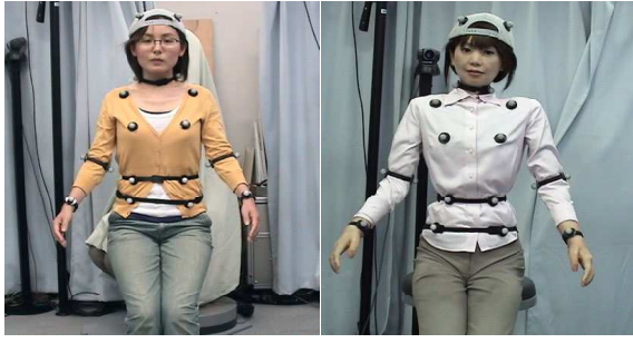
Fig. 6. The subject's postures mapped onto the android (taking a deep breath, \delta_e = 21.6\text{mm} , \sigma_s = 5.5\text{mm} ).
