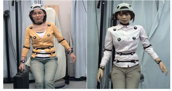
Fig. 8. The subject's postures mapped onto the android (holding heavy baggage, \delta_e = 36.1\text{mm} , \sigma_s = 12.8\text{mm} ).
