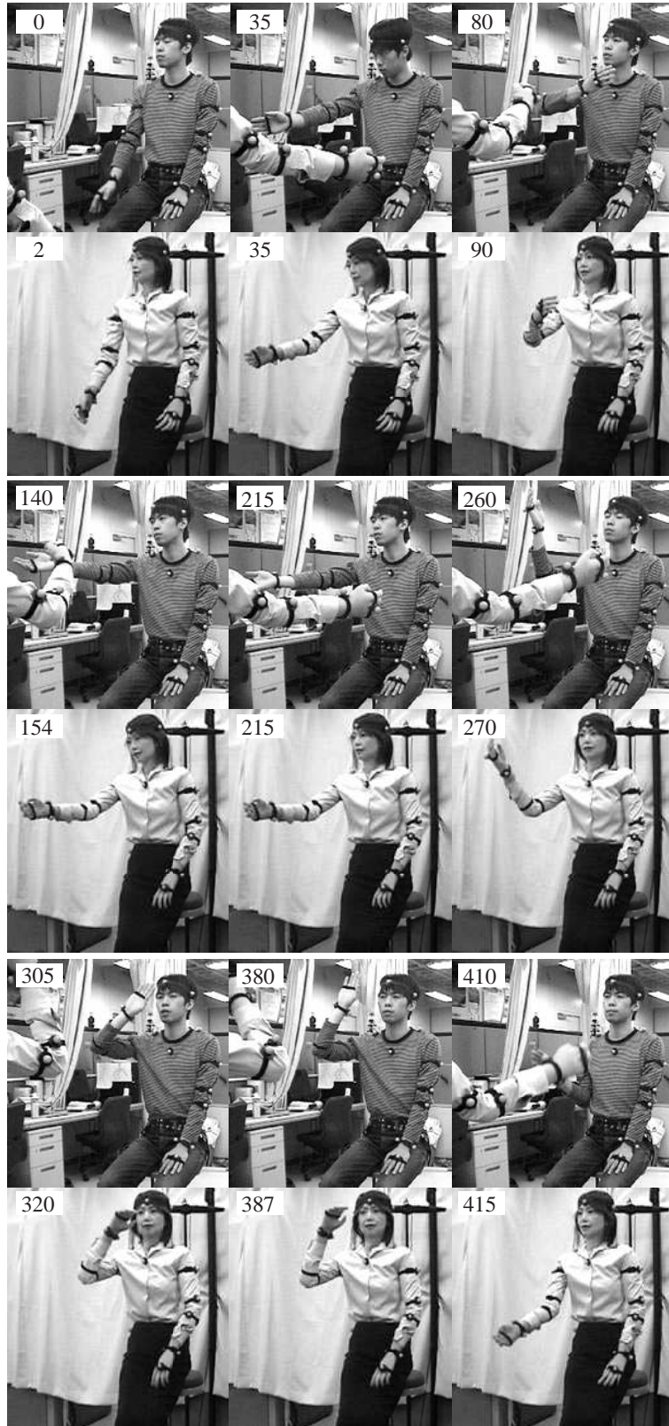
Figure 12: The generated android's motion compared to the subject's motion. The number represents the step.
