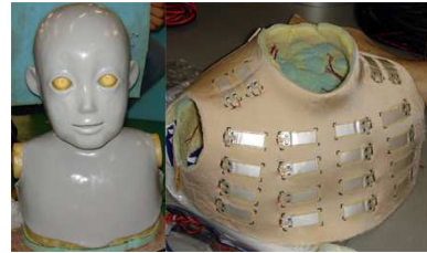
Fig.3 The silicone skin and tactile sensors.
