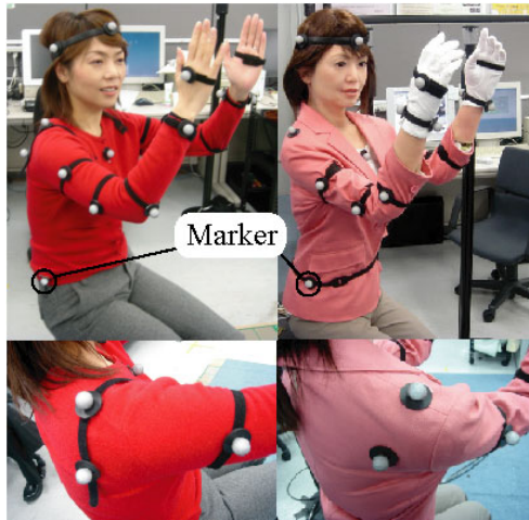
Figure 6: Marker positions on the master (left) and android (right)
