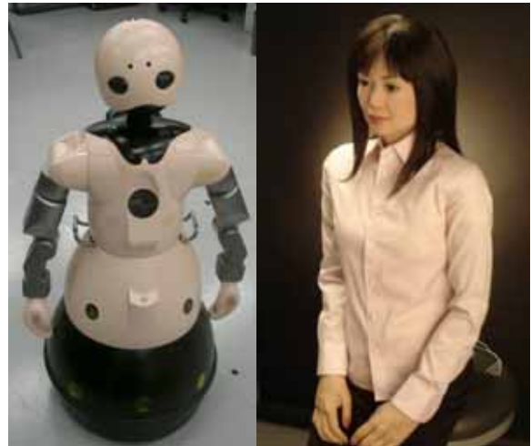
Figures 1: Humanoid and Android. The left picture shows a humanoid Eveliece P1 in Osaka University based on WAKAMARU that was developed by Mitsubishi Heavy Industry Co. Ltd.; and the right one shows an android Repliee Q2 developed by cooperation with KOKORO Co. Ltd. in Osaka University.
