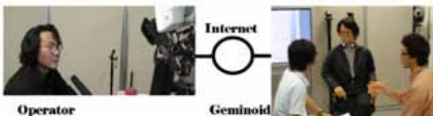
Figure 3: Myself, the geminoid, and the tele-operation system. The geminoid has been developed in ATR Intelligent Robotics and Communications Laboratories.
